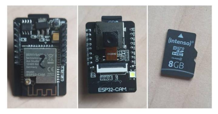
Fig 2. ESP32-Cam Al-Thinker + 8Gb SD Card
