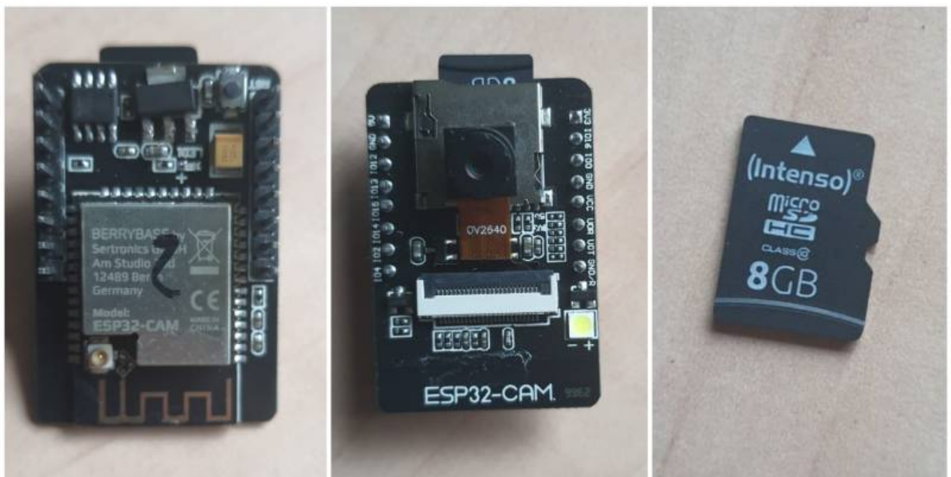
Fig 2. ESP32-Cam AI-Thinker + 8Gb SD Card
