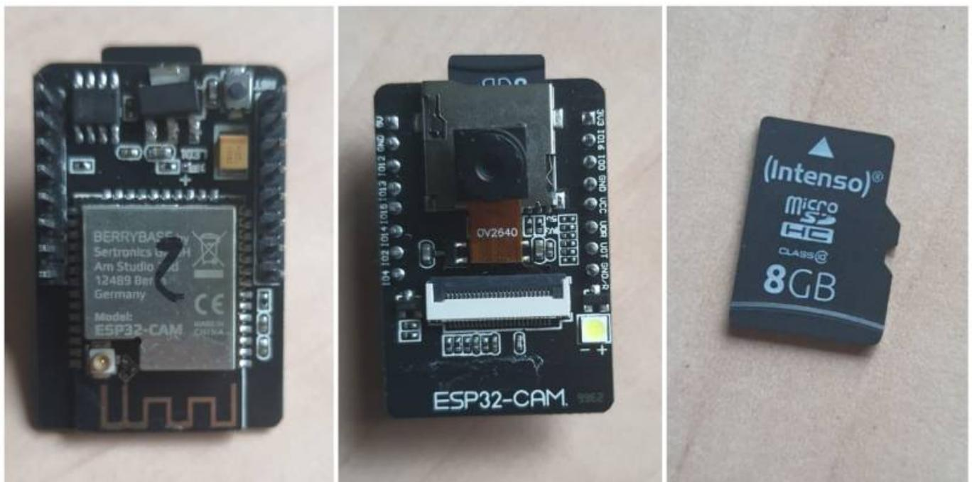
Fig 2. ESP32-Cam AI-Thinker + 8Gb SD Card
