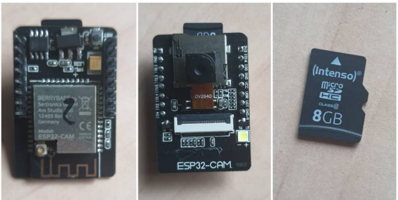
Fig 2. ESP32-Cam AI-Thinker + 8Gb SD Card
