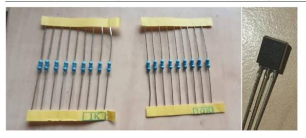
Fig 6. 1K, 10K resistors and 2N2222A NPN Transistor
