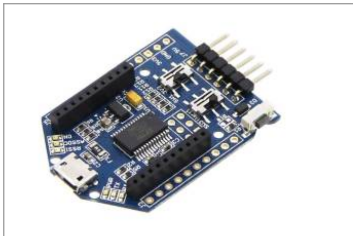
Figure 2. UartSBee v5.0 Module
