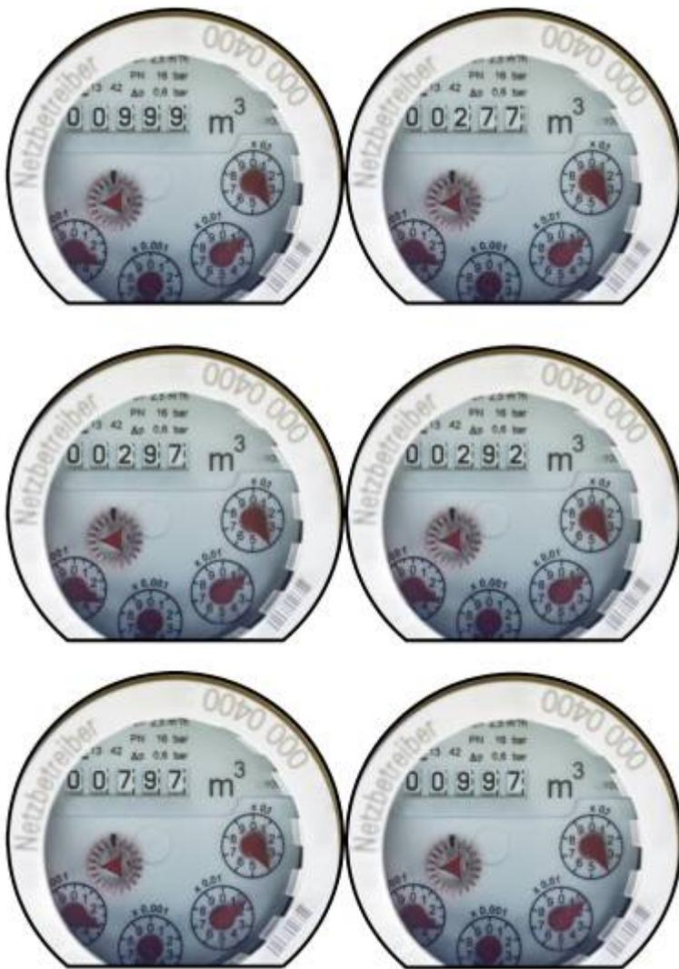
**Figure 8.** Sample images of watermeter with different readings
