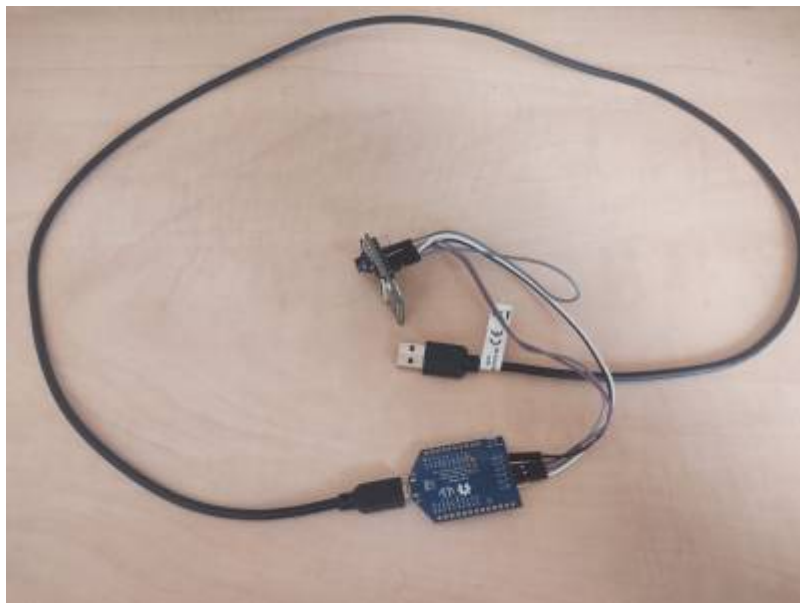
Figure 6. ESP32-CAM and Programmer connection with USB-A Cable
