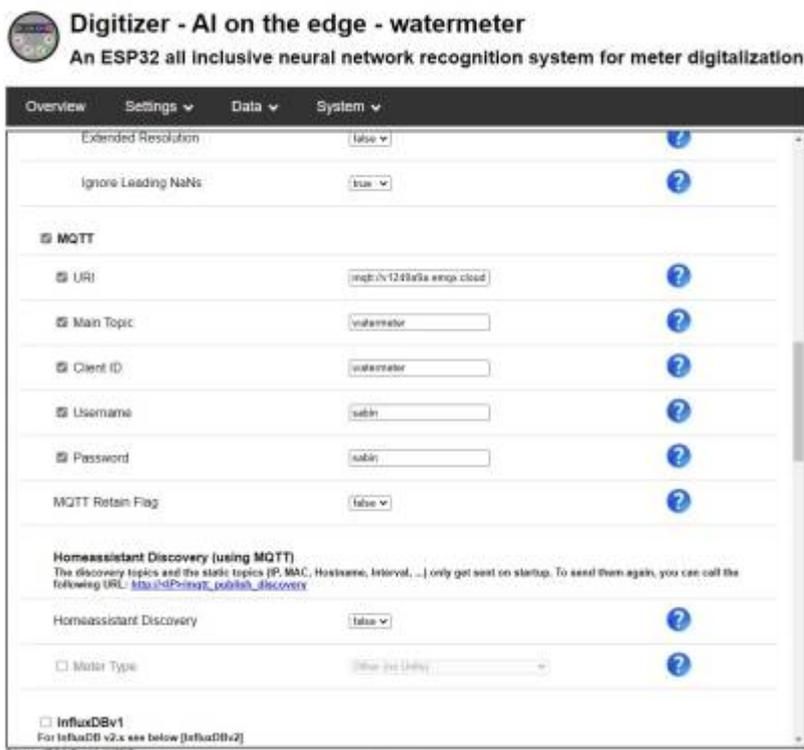
Figure 17. MQTT setup in the device software
