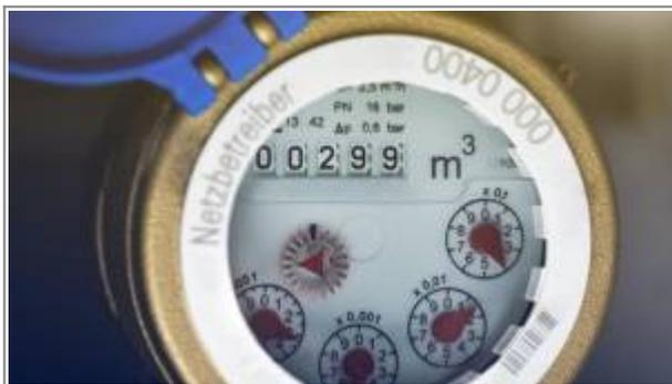
**Figure 3.** Example Watermeter
