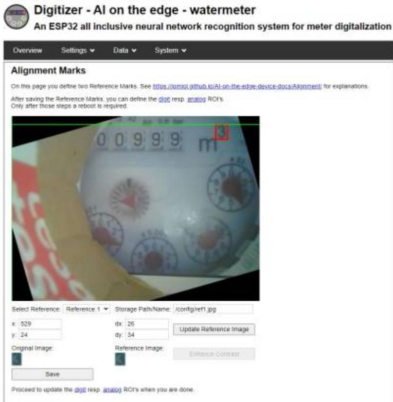
Figure 10. Alignment marks setup for 'm' and '3' as constant reference position
