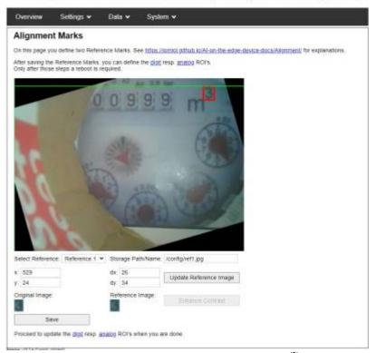
Figure 10. Alignment marks setup for 'm' and '3' as constant reference position
