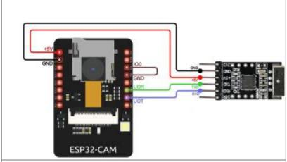
Figure 5. ESP32-CAM and Programmer connection Sketch
