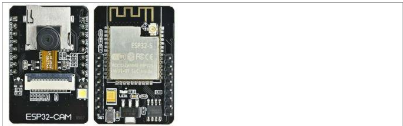
Figure 1. ESP32-CAM Source: https://www.nutsvolts.com/magazine/article/build-a-video-camera-using-the-esp32-cam-board
