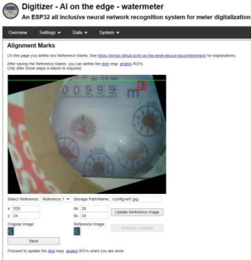
Figure 10. Alignment marks setup for 'm' and '3' as constant reference position
