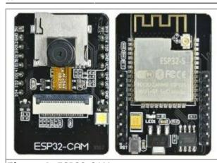
Figure 1. ESP32-CAM
