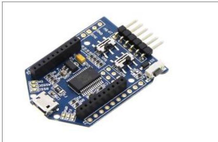
Figure 2. UartSBee v5.0 Module
