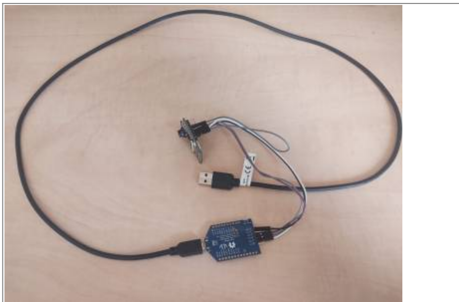
Figure 6. ESP32-CAM and Programmer connection with USB-A Cable
