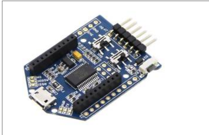
Figure 2. UartSBee v5.0 Module
