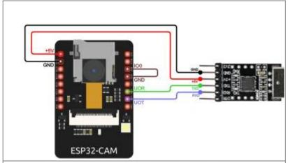
Figure 5. ESP32-CAM and Programmer connection Sketch
