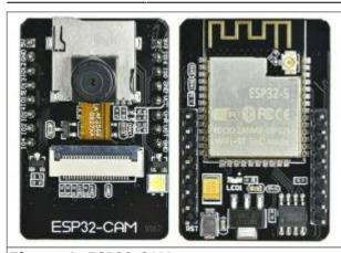
Figure 1. ESP32-CAM
