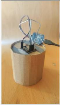
Figure 4 (b). Housing with the ESP32-CAM
