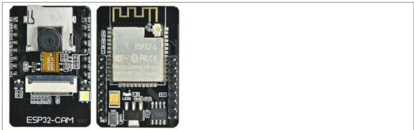
Figure 1. ESP32-CAM Source: https://www.nutsvolts.com/magazine/article/build-a-video-camera-using-the-esp32-cam-board
