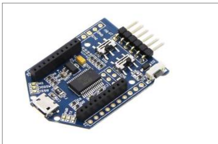
Figure 2. UartSBee v5.0 Module Source: https://wiki.seeedstudio.com/UartSBee_v5/
