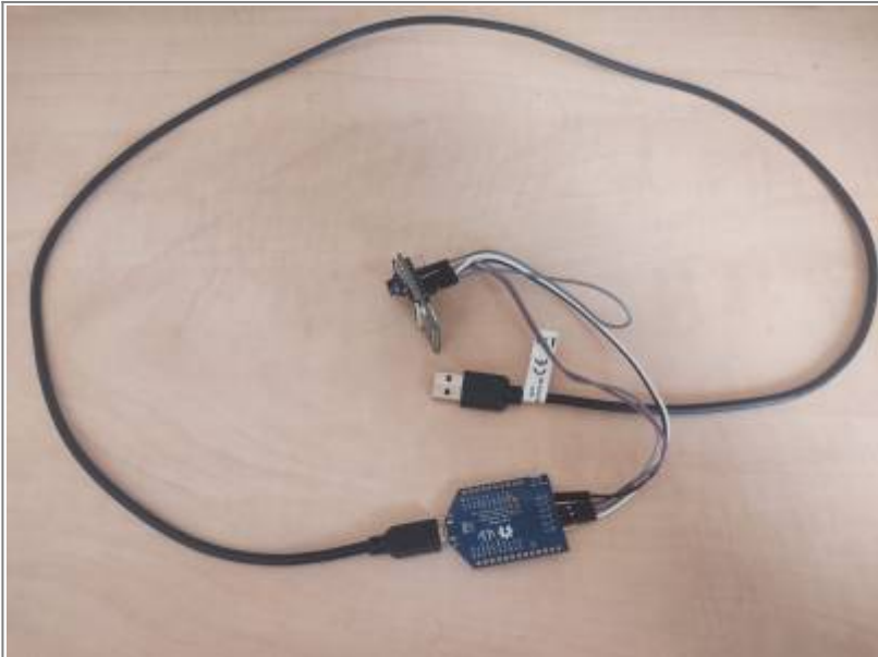
Figure 6. ESP32-CAM and Programmer connection with USB-A Cable
