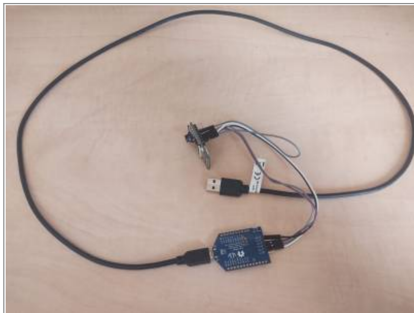
Figure 6. ESP32-CAM and Programmer connection with USB-A Cable
