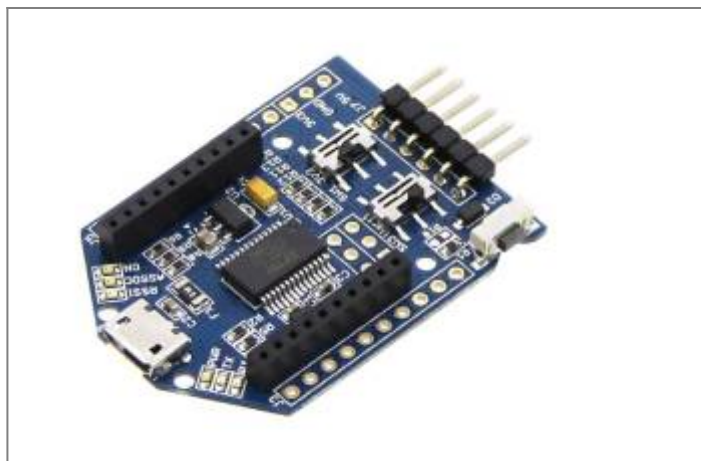
Figure 2. UartSBee v5.0 Module
