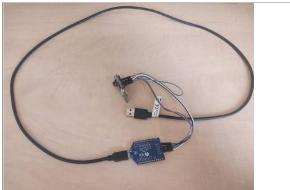
Figure 6. ESP32-CAM and Programmer connection with USB-A Cable
