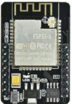
Figure 1. ESP32-CAM
