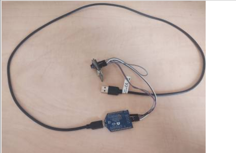
Figure 6. ESP32-CAM and Programmer connection with USB-A Cable
