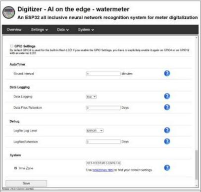
Figure 15. Interval and data retention configuration
