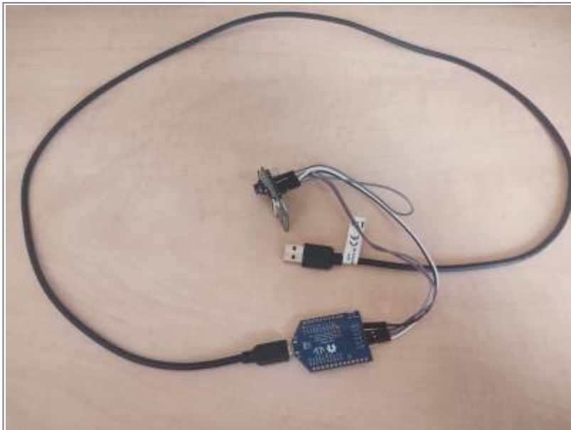
Figure 6. ESP32-CAM and Programmer connection with USB-A Cable
