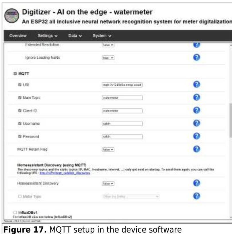
**Figure 17.** MQTT setup in the device software
