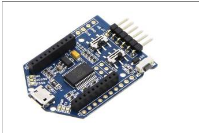
Figure 2. UartSBee v5.0 Module
