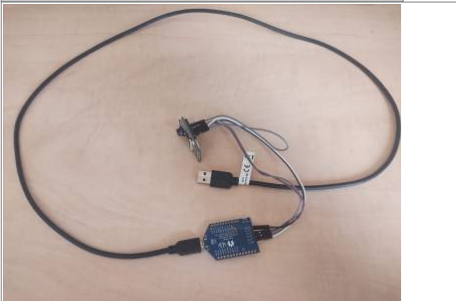
Figure 6. ESP32-CAM and Programmer connection with USB-A Cable
