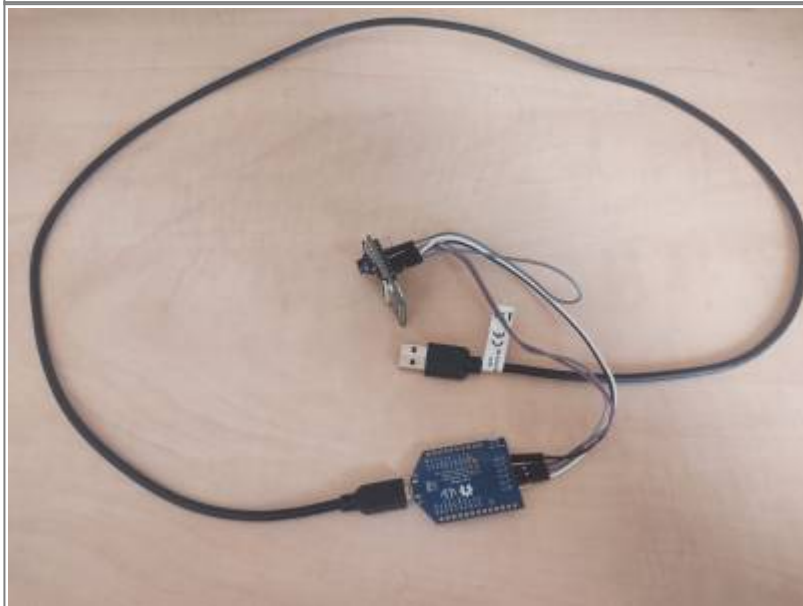
Figure 6. ESP32-CAM and Programmer connection with USB-A Cable
