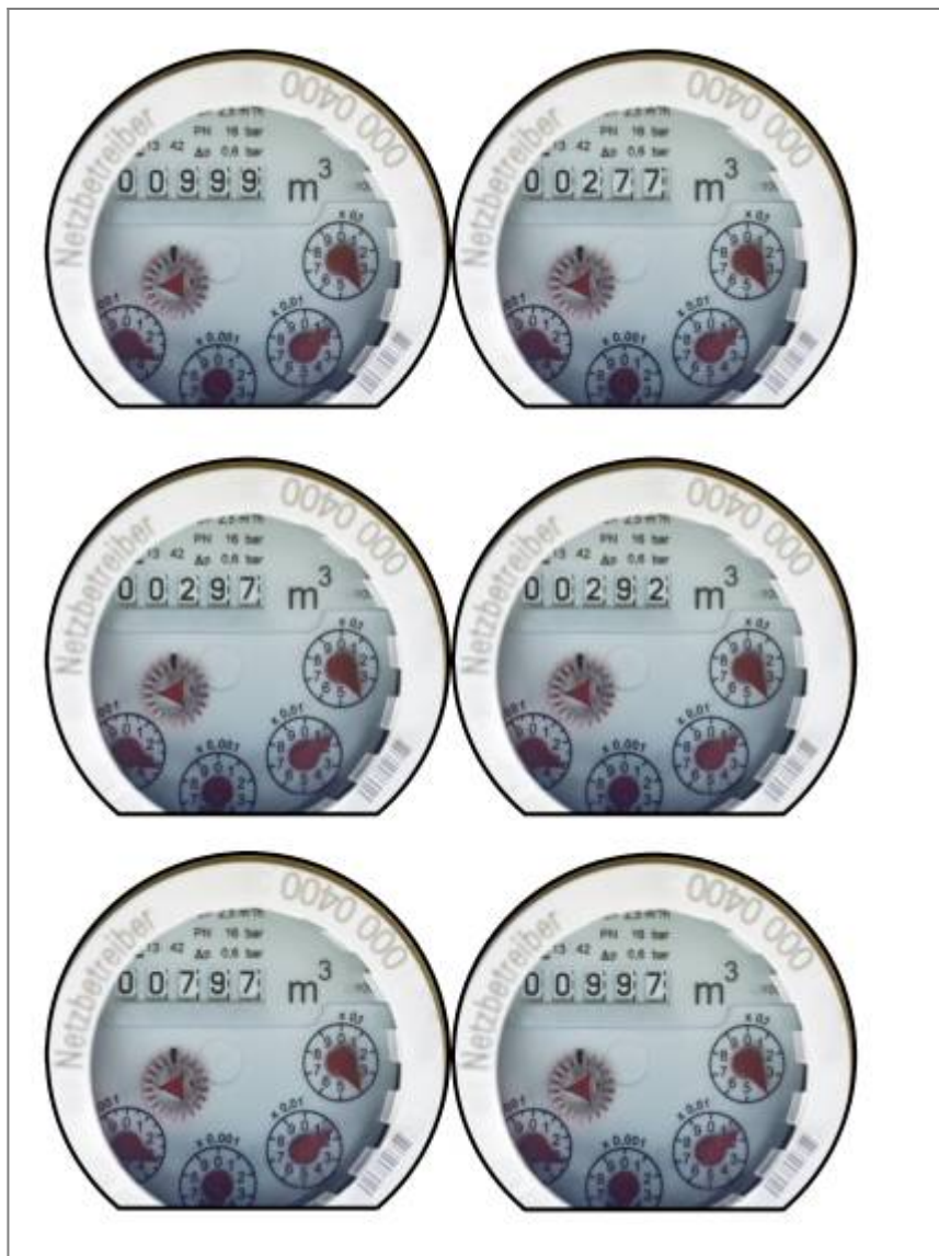
Figure 8. Sample images of watermeter with different readings
