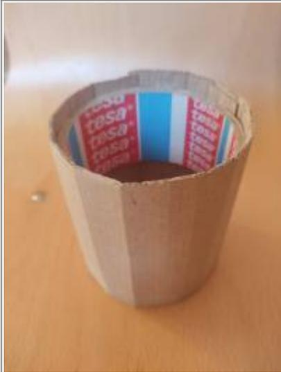
**Figure 4 (a).** Housing without the ESP32-CAM
