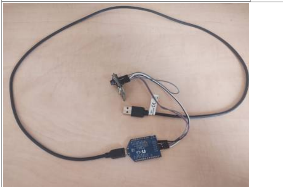
Figure 6. ESP32-CAM and Programmer connection with USB-A Cable
