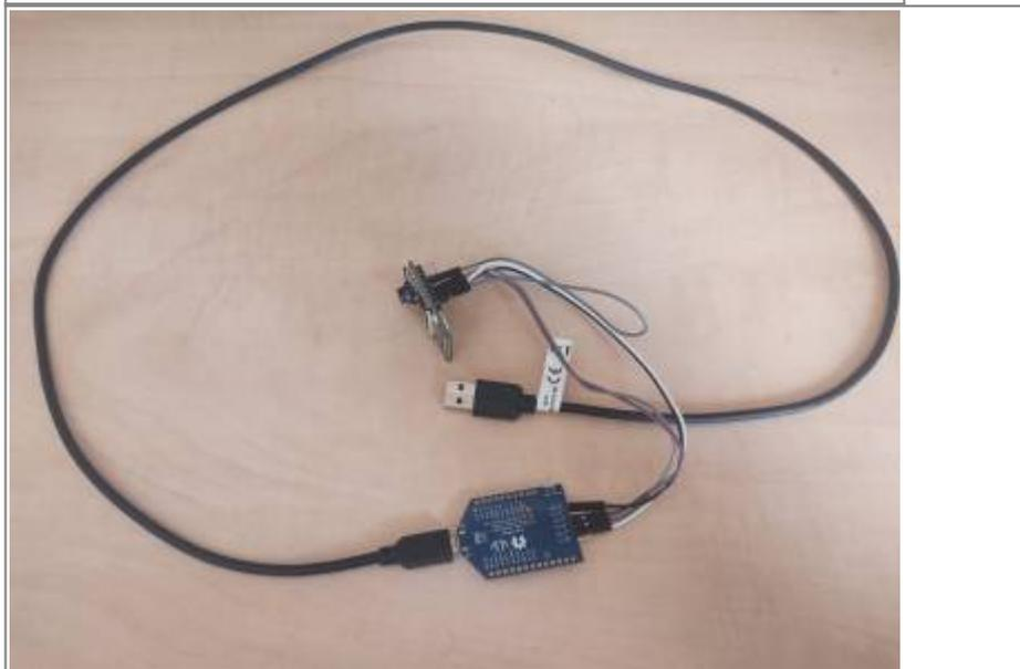
**Figure 6.** ESP32-CAM and Programmer connection with USB-A Cable
