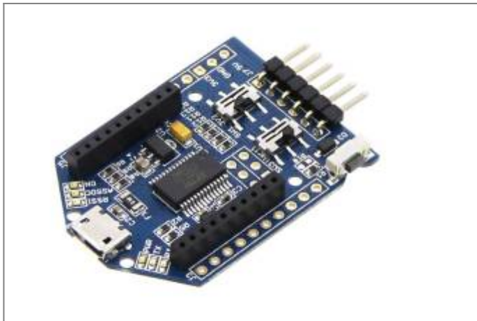
Figure 2. UartSBee v5.0 Module
