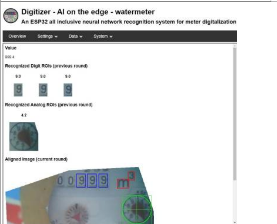
Figure 14. (a) Device reading the reference image as a sample image
