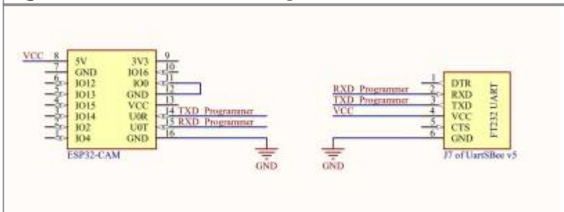
**Figure 7.** Schematic drawing of connection for programming
