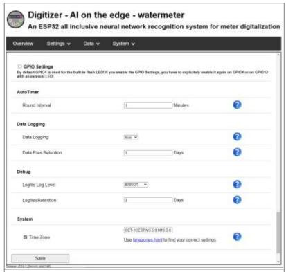
Figure 15. Interval and data retention configuration
