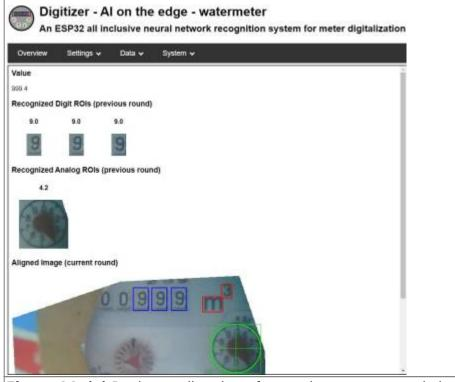
Figure 14. (a) Device reading the reference image as a sample image
