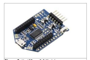
**Figure 2.** UartSBee v5.0 Module Source: https://wiki.seeedstudio.com/UartSBee v5/
