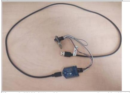
Figure 6. ESP32-CAM and Programmer connection with USB-A Cable
