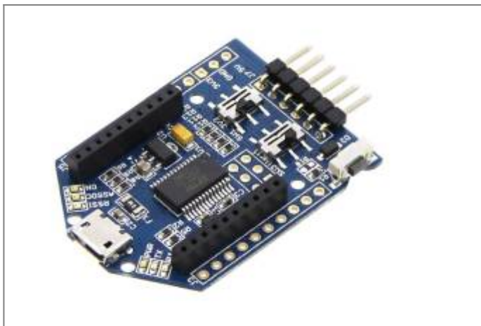
Figure 2. UartSBee v5.0 Module
