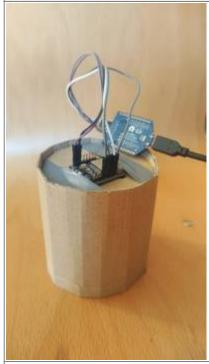
Figure 4 (b). Housing with the ESP32-CAM
