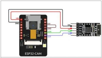
Figure 5. ESP32-CAM and Programmer connection Sketch
