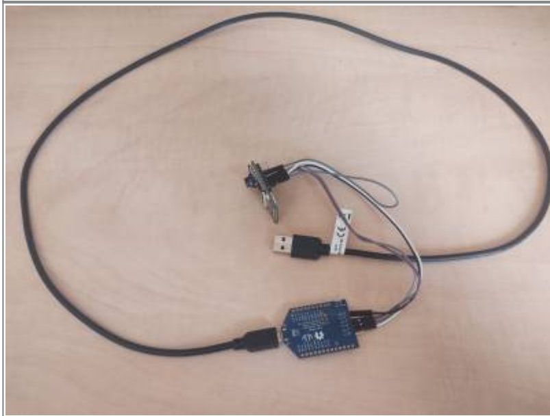
Figure 6. ESP32-CAM and Programmer connection with USB-A Cable
