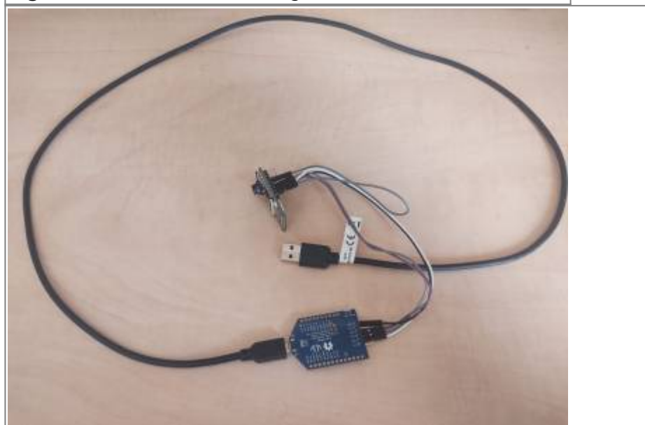
Figure 6. ESP32-CAM and Programmer connection with USB-A Cable
