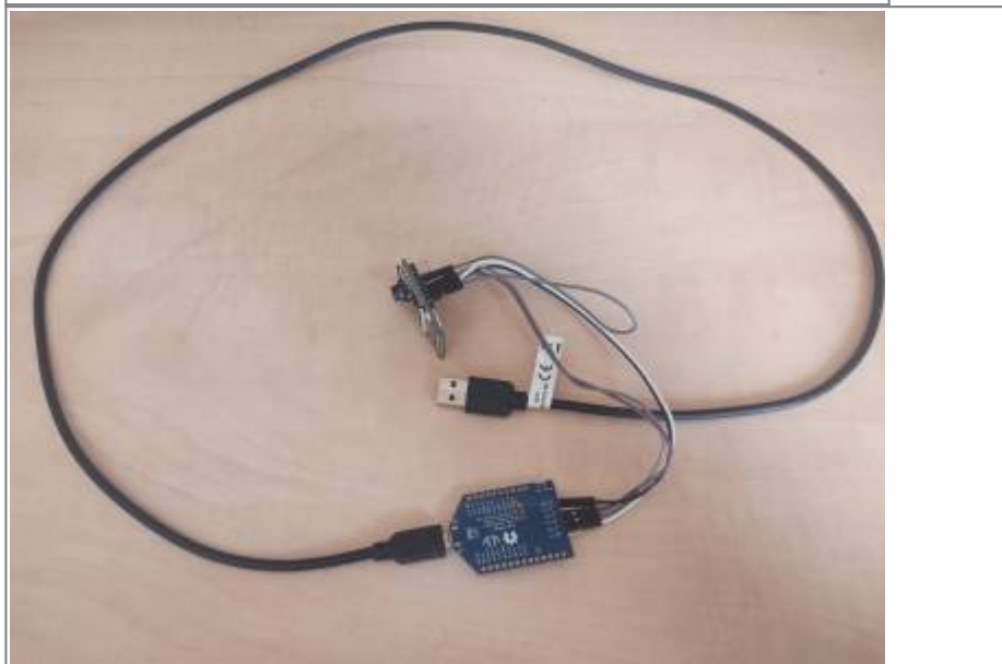
Figure 6. ESP32-CAM and Programmer connection with USB-A Cable
