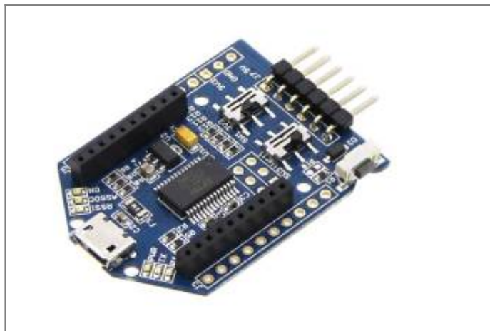
Figure 2. UartSBee v5.0 Module
