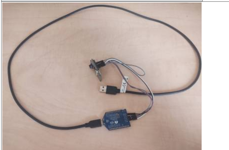
Figure 6. ESP32-CAM and Programmer connection with USB-A Cable
