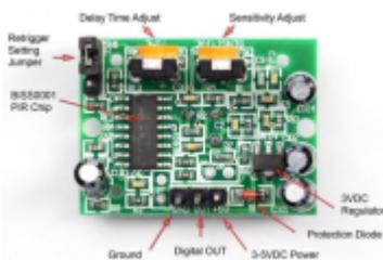
Fig 5: PIR sensor description (source: Adafruit )
