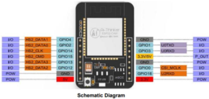
Pins configuration on Esp32cam module
