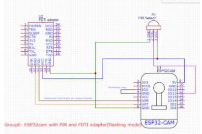
Fig3: Esp32 cam on flashing mode(
