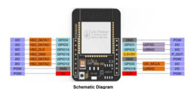
Fig2: Pins configuration on Esp32cam
