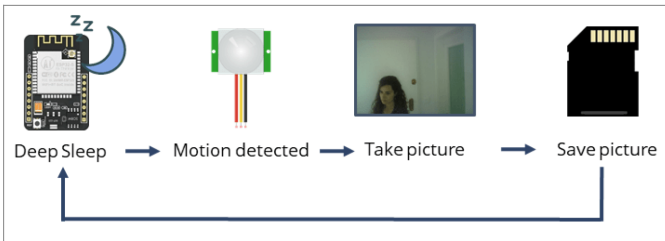
Figure 9. The process from detecting movement to deep sleep mode
