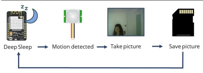
Deep sleep mode of the ESP32 reduces the amount of power consumed while in operation, but enough power is left to keep the processor and RTC peripherals running. When in deep sleep mode, the CPU, Wi-Fi and bluetooth are disabled. This power-saving feature is quite useful in extending the battery life. When the ESP32 camera is stimulated, in this case by the motion sensor, it will wake up and function as normal.
