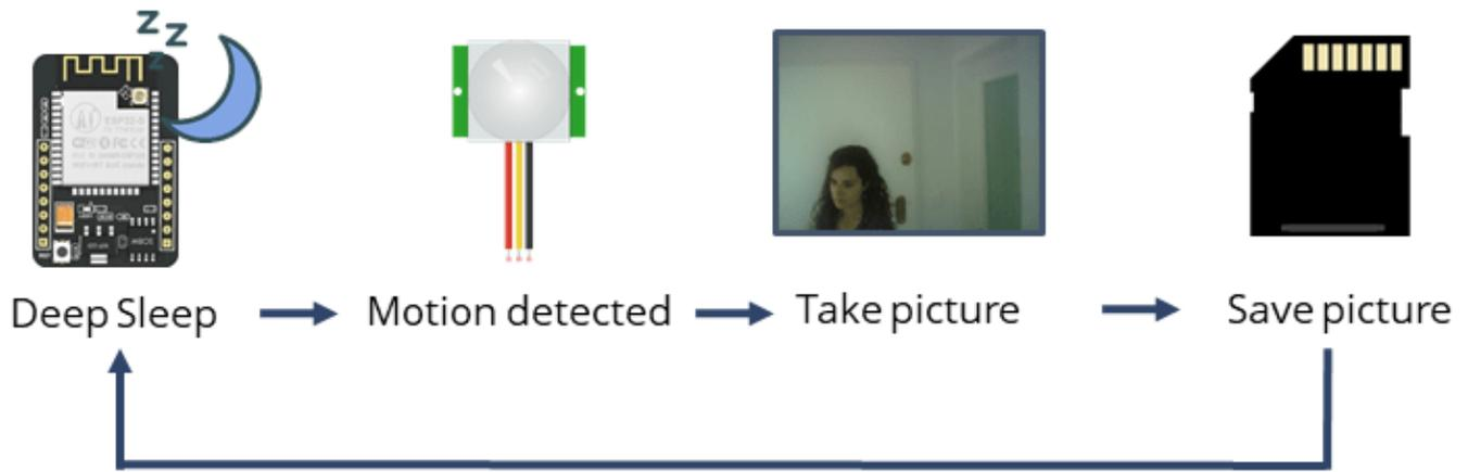
Deep sleep mode of the ESP32 reduces the amount of power consumed while in operation, but enough power is left to keep the processor and RTC peripherals running. When in deep sleep mode, the CPU, Wi-Fi and bluetooth are disabled. This power-saving feature is quite useful in extending the battery life. When the ESP32 camera is stimulated, in this case by the motion sensor, it will wake up and function as normal.
