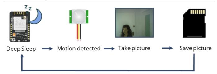
Deep sleep mode of the ESP32 reduces the amount of power consumed while in operation, but enough power is left to keep the processor and RTC peripherals running. When in deep sleep mode, the CPU, Wi-Fi and bluetooth are disabled. This power-saving feature is quite useful in extending the battery life. When the ESP32 camera is stimulated, in this case by the motion sensor, it will wake up and function as normal.
