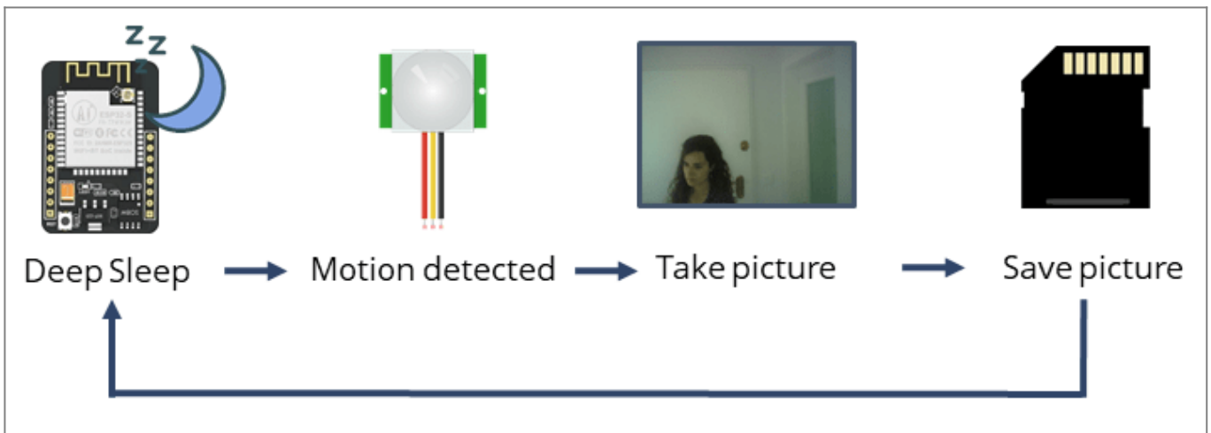
Figure 9. The process from detecting movement to deep sleep mode
