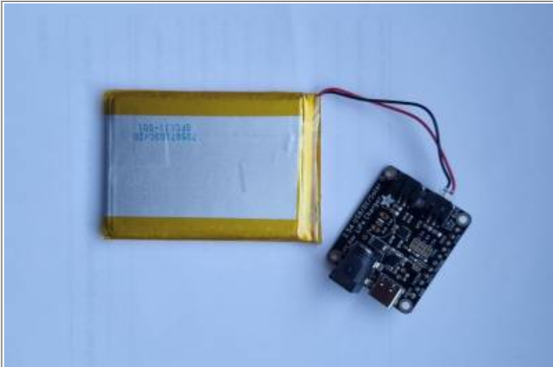
Figure 6. 1.5 USB/DC/Solar LiPo Charger
