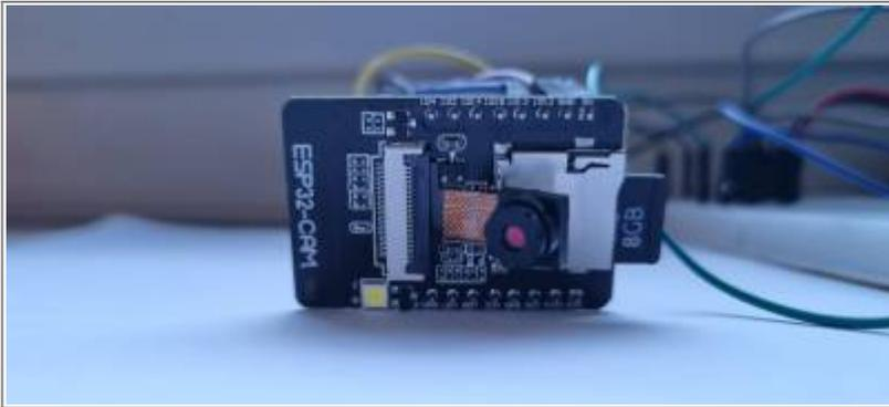
**Figure 3.** ESP32 camera
