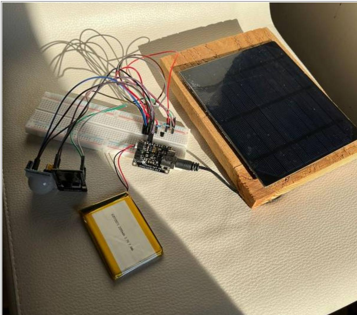
**Figure 1.** Complete setup of smart bird house
