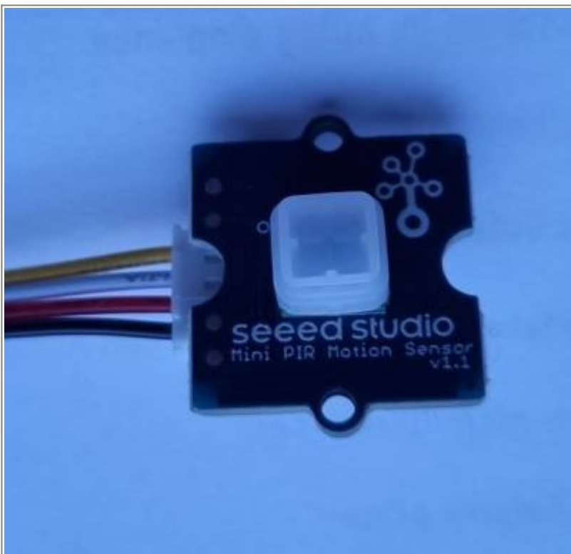
Figure 4. Seeed Studio mini PIR motion sensor
