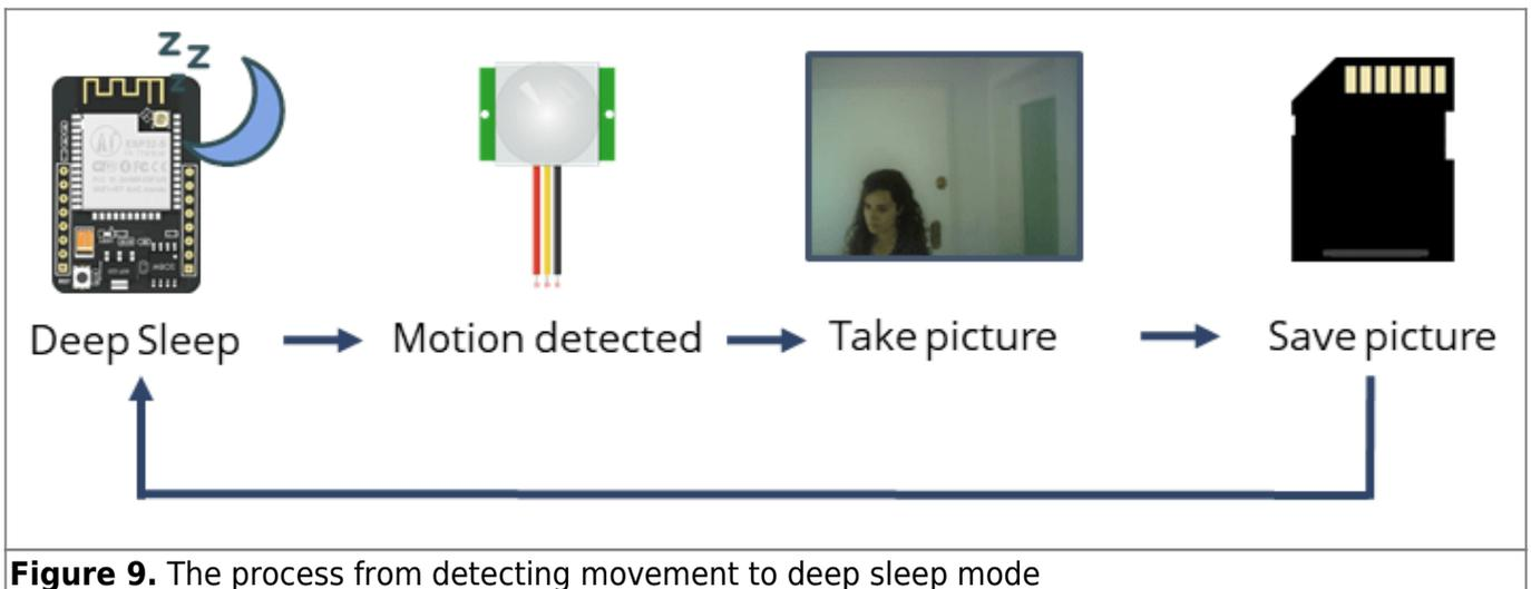
**Figure 9.** The process from detecting movement to deep sleep mode
