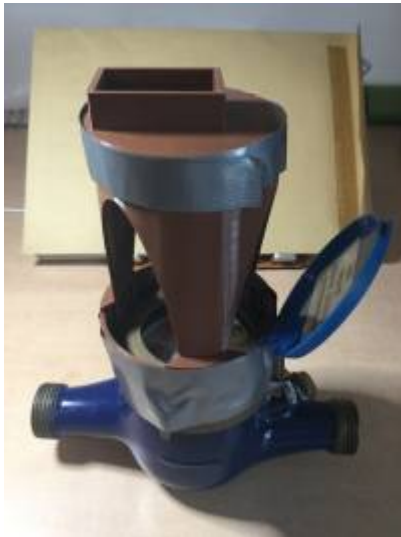
Figure 11: ESP32CAM and watermeter casing
