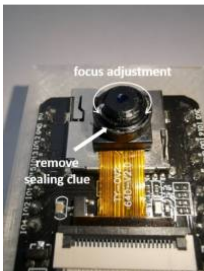
Figure 10: Focus adjustment of the camera
