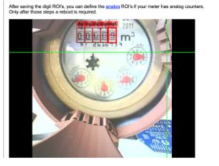
To adjust the positions of the ROIs within the reading, we used the options "Move Next" or "Move Previous." Finally, we saved all our changes with "Save all to Config.ini."Since our water meter lacked analog information, we unchecked the next step.
