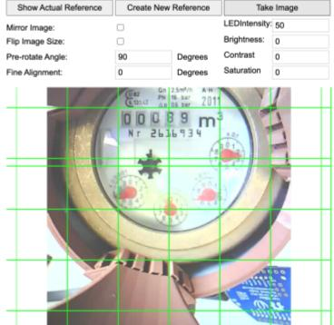
However, we encountered an issue with the ESP32's built-in LED, as its flashing caused unwanted reflections on the glass of the water meter, making the Al-based readout challenging. To address this, we decided to cover the LED with a piece of tape, which provided better control over reflections and
