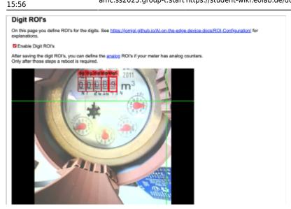
To adjust the positions of the ROIs within the reading, we used the options "Move Next" or "Move Previous." Finally, we saved all our changes with "Save all to Config.ini." Since our water meter lacked analog information, we unchecked the next step.
