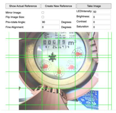
However, we encountered an issue with the ESP32's built-in LED, as its flashing caused unwanted reflections on the glass of the water meter, making the AI-based readout challenging. To address this, we decided to cover the LED with a piece of tape, which provided better control over reflections and
