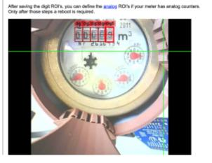
To adjust the positions of the ROIs within the reading, we used the options "Move Next" or "Move Previous." Finally, we saved all our changes with "Save all to Config.ini." Since our water meter lacked analog information, we unchecked the next step.
