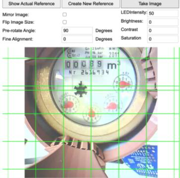
However, we encountered an issue with the ESP32's built-in LED, as its flashing caused unwanted reflections on the glass of the water meter, making the Al-based readout challenging. To address this, we decided to cover the LED with a piece of tape, which provided better control over reflections and
