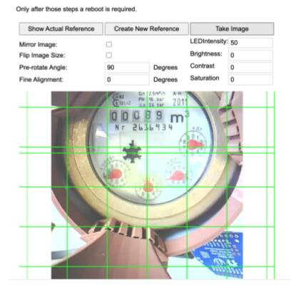
However, we encountered an issue with the ESP32's built-in LED, as its flashing caused unwanted reflections on the glass of the water meter, making the Al-based readout challenging. To address this, we decided to cover the LED with a piece of tape, which provided better control over reflections and improved the accuracy of the readings.
