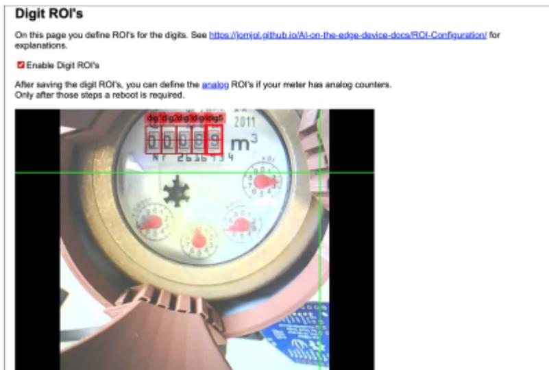
To adjust the positions of the ROIs within the reading, we used the options “Move Next” or “Move Previous.” Finally, we saved all our changes with “Save all to Config.ini.” Since our water meter lacked analog information, we unchecked the next step.
