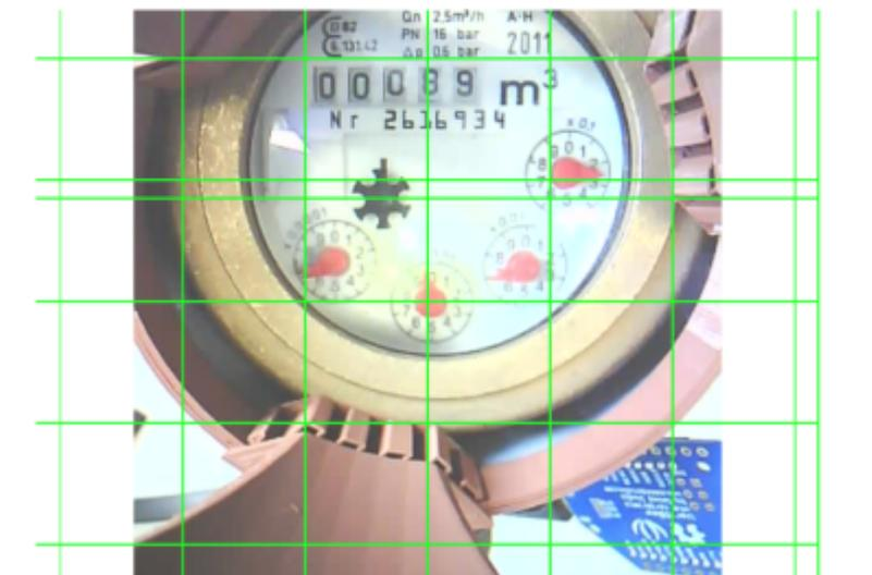
However, we encountered an issue with the ESP32's built-in LED, as its flashing caused unwanted reflections on the glass of the water meter, making the AI-based readout challenging. To address this, we decided to cover the LED with a piece of tape, which provided better control over reflections and improved the accuracy of the readings.
