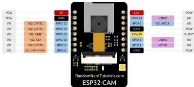
Figure 2: ESP32CAM pinout https://randomnerdtutorials.com/esp32-cam-video-streaming-face-recognition-arduino-ide/
