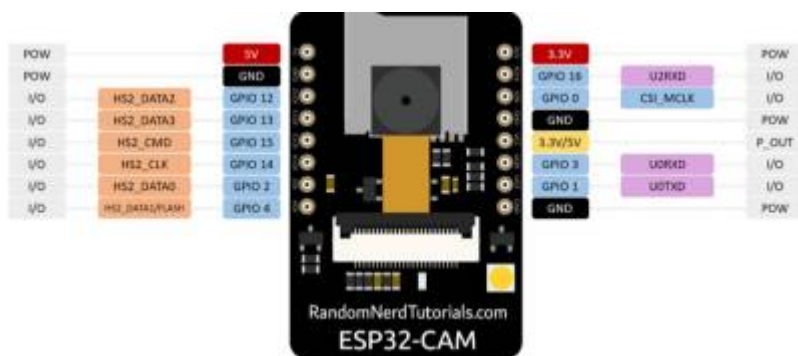
Figure 2: ESP32CAM pinout https://randomnerdtutorials.com/esp32-cam-video-streaming-face-recognition-arduino-ide/
