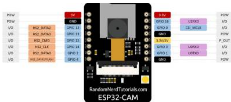
Figure 2: ESP32CAM pinout
