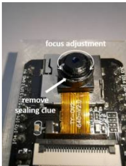
Figure 10: Focus adjustment of the camera
