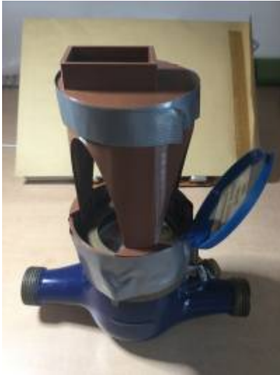
Figure 11: ESP32CAM and watermeter casing
