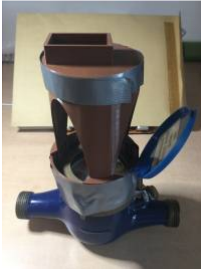
Figure 11: ESP32CAM and watermeter casing
