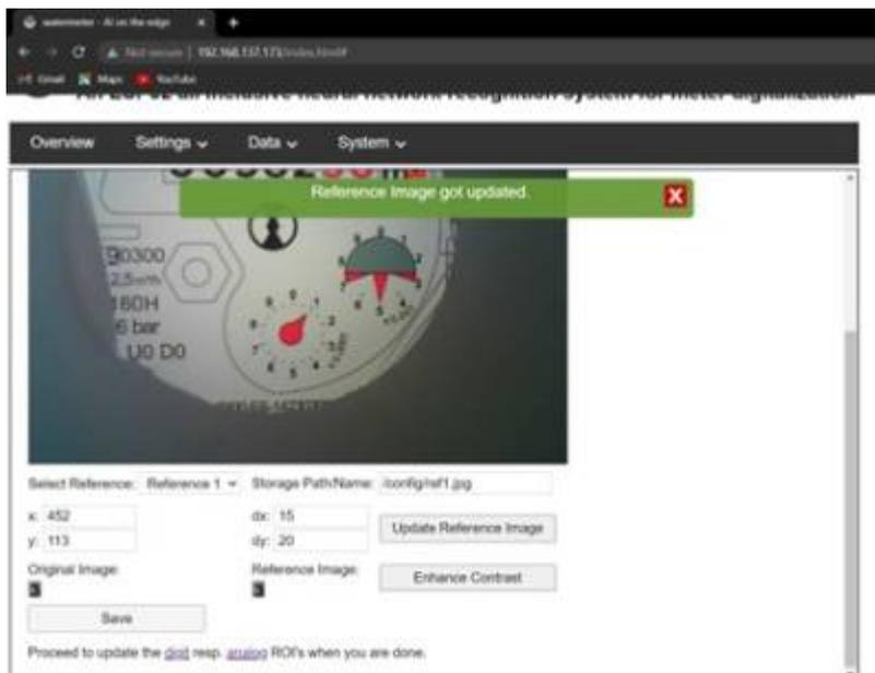
Fig 13: Updating the reference. Source: own image - Shreevarshan
