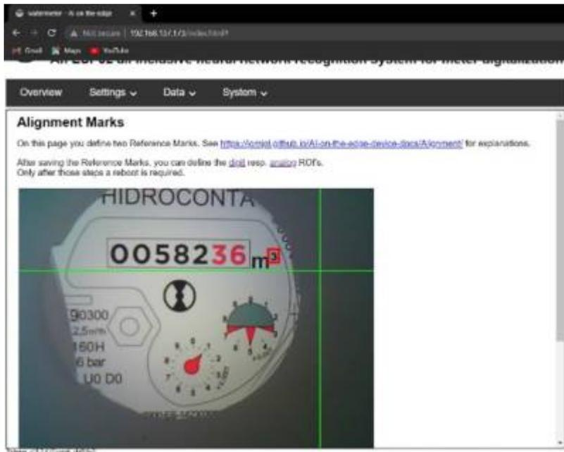
Fig 12: Creating Alignment marks. Source: own image- Shreevarshan
