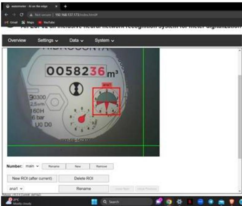
Fig 15: Referencing the analogs. Source: own image - Shreevarshan
