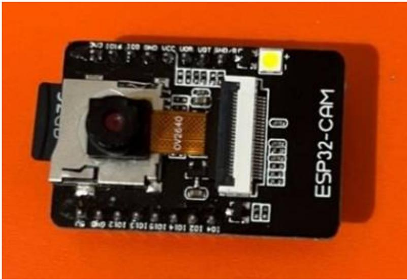
Fig1: ESP-32 module. Source: own image - Shreevarshan
