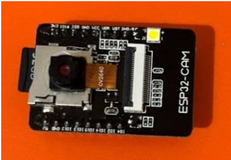
Fig1: ESP-32 module. Source: own image - Shreevarshan
