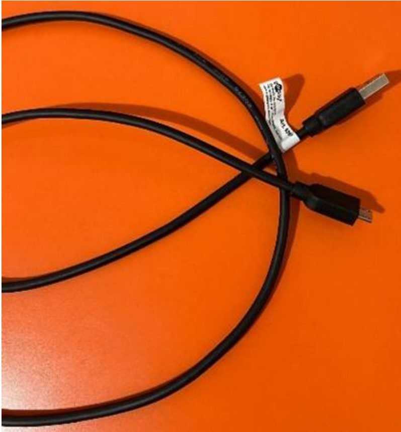
Fig 3: Micro USB to USB-A. Source: own image - Shreevarshan
