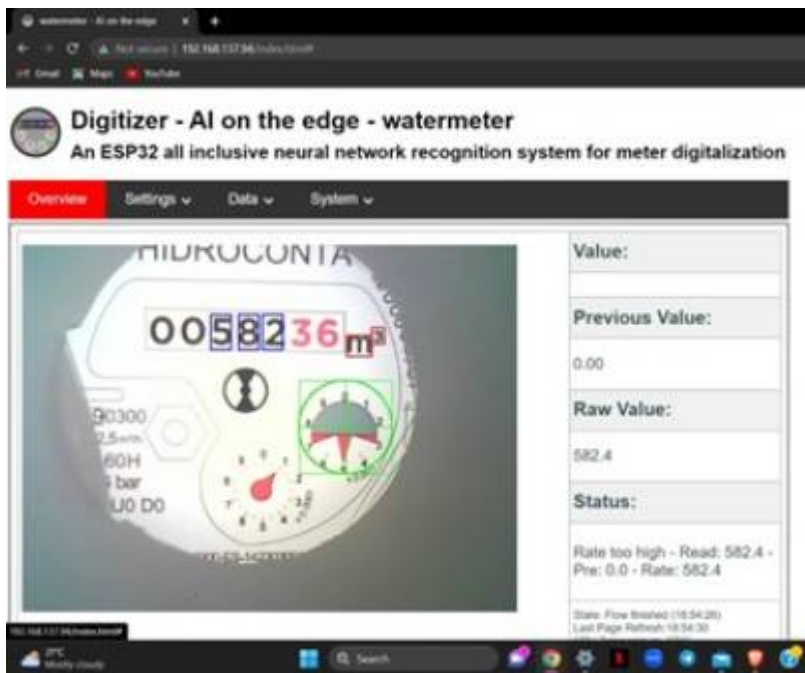
Fig 16: Final reading of the values in the water meter reference. Source: own image - Shreevarshan
