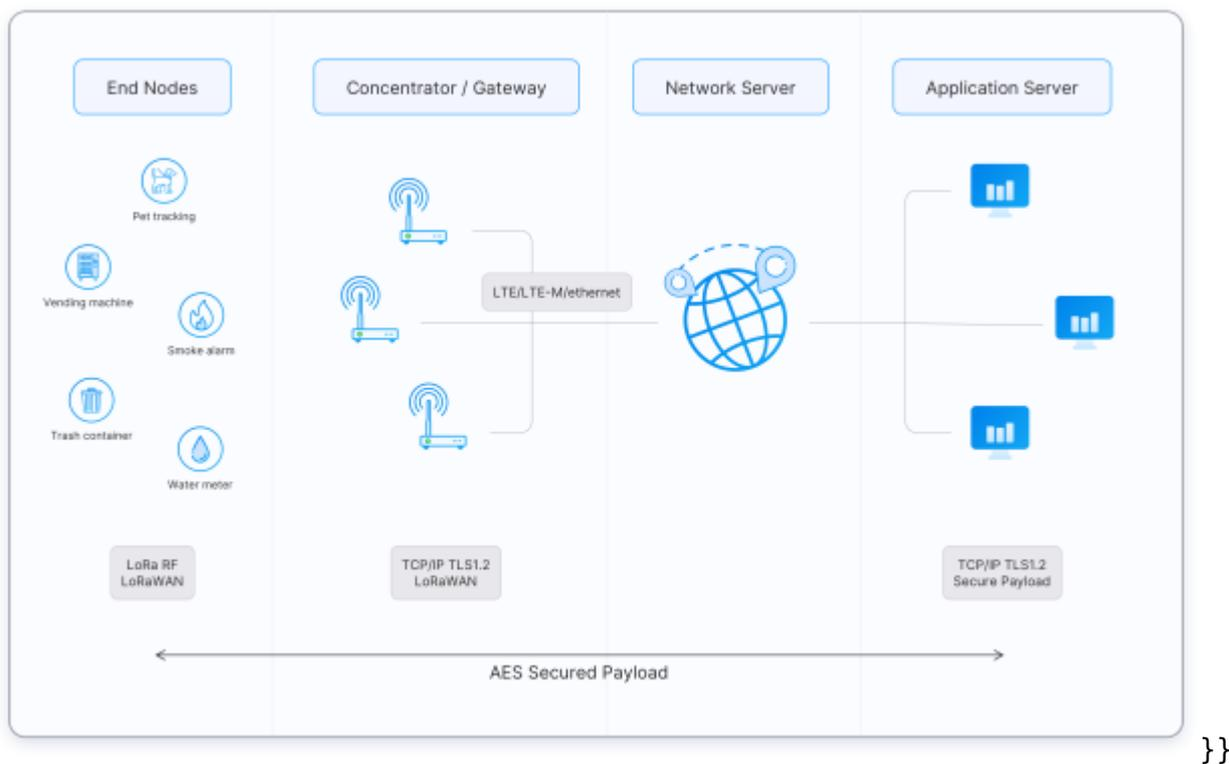
Fig.8, Elements in a typical LoRaWAN network, Source: <https://www.thethingsnetwork.org/docs/lorawan/architecture/>
