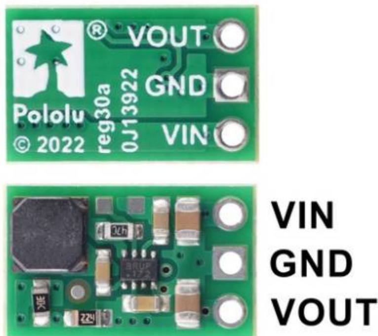
Fig.5, Voltage Regulator, Source: https://www.pololu.com/product/4945
