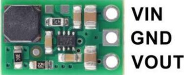
Fig.5, Voltage Regulator, Source: https://www.pololu.com/product/4945
