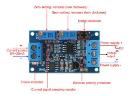
Fig.4, Current to Voltage Converter, Source: https://www.robotics.org.za/XY-ITOV
