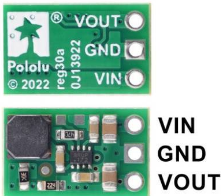
Fig.5, Voltage Regulator, Source: https://www.pololu.com/product/4945
