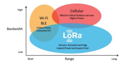
Fig.7, LoRa comparisson with other wireless data transmission technologies, Source:
