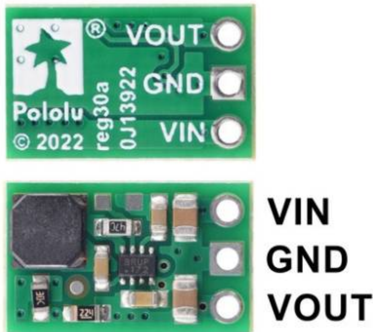
Fig.5, Voltage Regulator, Source: https://www.pololu.com/product/4945
