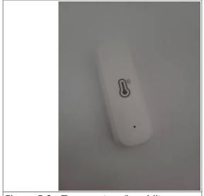
Figure 5.2 - Temperature/humidity sensor
