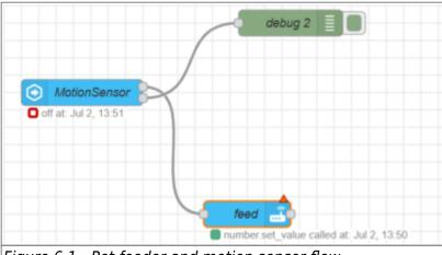
Figure 6.1 - Pet feeder and motion sensor flow
