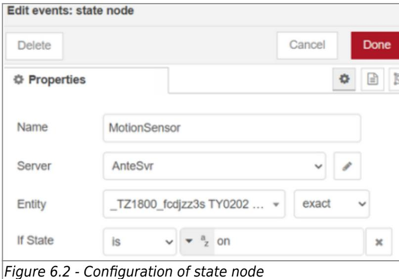
Figure 6.2 - Configuration of state node
