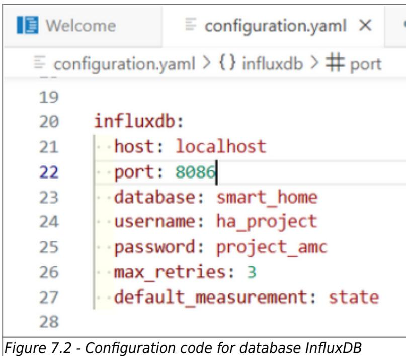
Figure 7.2 - Configuration code for database InfluxDB
