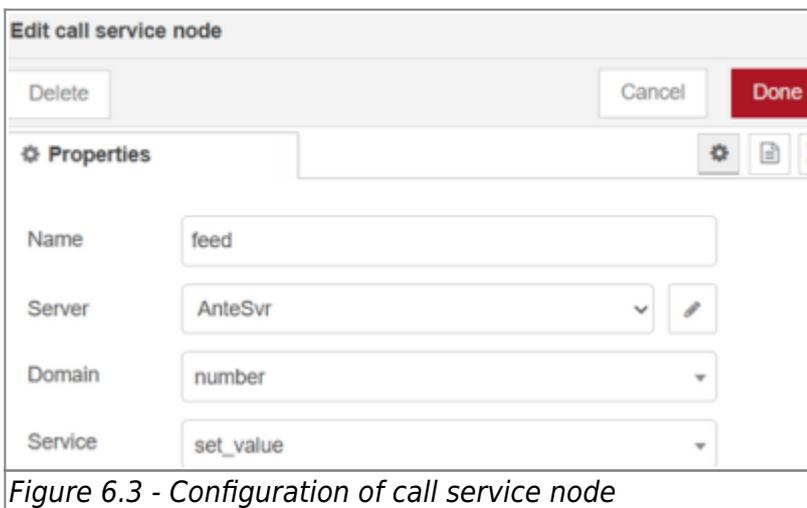
Figure 6.3 - Configuration of call service node
